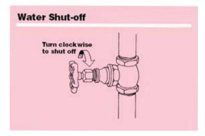
Shut off the main valve to prevent contamination of the water supply in your water heater and plumbing.
