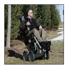
The 4-Wheel Function enables the user to climb curbs as high as five inches and to travel over a variety of uneven terrain, such as sand, gravel, grass, thick carpet and other surfaces.
